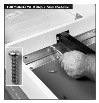
Finger tighten the top's foot end to frame using 4 silver, 1/4-20 x 1" truss head screws and 5/16" washers. Slide the foot end toward the center board and finish tightening screws.
