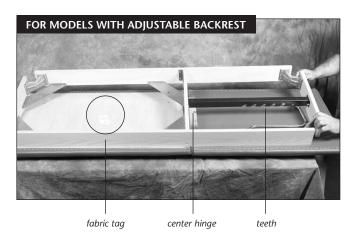
Align the holes in the hinge with the holes in the center board and fasten to center board using 4 silver, 1/4-20 x 1" truss head screws.
