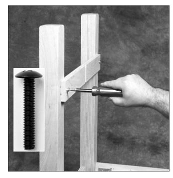
Position the spanner finished edge towards top and align the hole in the center of the spanner with the hole in the H-brace and finger tighten on one end then repeat on the opposite end using the #8 screws. Finish by tightening both ends. **DO NOT OVER TIGHTEN.**
