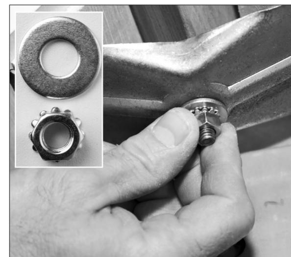
**5** Position the H-brace with finished edge toward top with the cut-out slot facing toward the inside of the table and attach using the 4 black 1/4-20 x 1 1/2" truss head screws.
