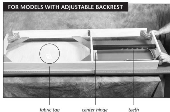
**2** Align the holes in the hinge with the holes in the center board and fasten to center board using 4 silver, 1/4-20 x 1" truss head screws.
