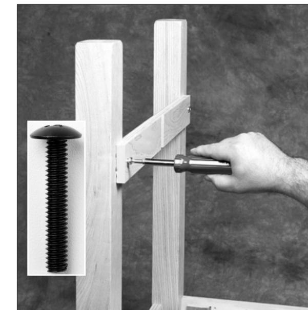
**6** Position the spanner finished edge towards top and align the hole in the center of the spanner with the hole in the H-brace and finger tighten on one end then repeat on the opposite end using the #8 screws. Finish by tightening both ends. **DO NOT OVER TIGHTEN.**
