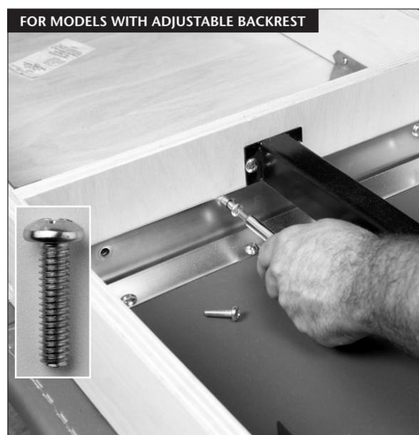
**3** Finger tighten the top's foot end to frame using 4 silver, 1/4-20 x 1" truss head screws and 5/16" washers. Slide the foot end toward the center board and finish tightening screws.
