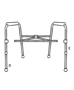
mode depress the push pins to release the cross brace for the frame of the commode.
